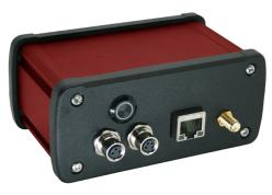
The ConnectPoint AP access point serves as the heart of the ConnectPoint system. It establishes the HaLow network . and controls the network parameters. It connects to a ConnectPoint Station or another ConnectPoint AP either • individually or simultaneously. One ConnectPoint AP is required in every network. It
