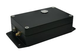
The SensePoint Motor node has three 1V CT channels and eight PT100 RTD channels. It is designed to verify the health of electric motors by monitoring the motor currents and temperatures of various components. It communicates with a Nexus gateway over a Wi-Fi HaLow or customized Thread wireless link.
