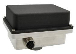
The SensePoint Accel node includes a three-axis accelerometer for vibration measurements in Condition Based Monitoring (CbM) applications. With a 6kHz bandwidth and 16g dynamic range, the SensePoint Accel is suitable for monitoring for bearing faults as well as imbalance and misalignment.
