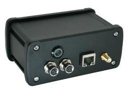
The ConnectPoint Station is an Specifications end point in the HaLow network. • It is a bridge between a HaLow network and both Ethernet and • RS-485 networks, automatically passing data between the networks. It communicates with a ConnectPoint AP to act as a cable replacement between end devices.
