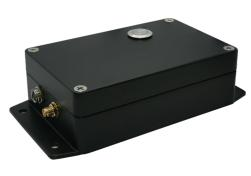
The SensePoint Industrial node Specifications offers 4 channels of 4-20mA analog inputs, 4 channels of 0-24V analog inputs and four channels that are 0-48V digital inputs. A single Dallas 1-Wire channel enables operation with • digital sensors. A 50V power input makes it compatible with 48V industrial systems. It communicates with a Nexus
