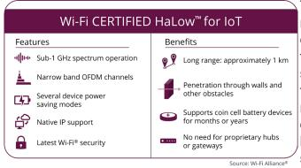
The 802.11ah specification or Wi-Fi HaLow, was released by the Wi-Fi Alliance in 2017. It is best described as "sub-GHz long-range Wi-Fi". It takes the features that have made Wi-Fi one of the most successful wireless protocols and brings it into lower frequency bands. It fills a gap by offering much better range than Bluetooth and IEEE 802.15.4 radios while offering much better data throughput than protocols like ZigBee, Thread and LoRa. This allows it to offer several distinct advantages.
