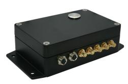
The Nexus Industrial gateway communicates with SensePoint nodes over Wi-Fi HaLow or a customized Thread wireless network. It uses a CAT-1 cellular modem to communicate with cloud servers.
