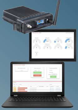
Nexcomm System's CAN-2-Cloud is a fully integrated solution that includes hardware, firmware, cellular data and web-based software in a single, cohesive system. The system accepts a list of CAN messages to be monitored and how often each one should be reported. The monitored messages are then pushed up to the cloud where the data are displayed, reported and graphed as desired.
