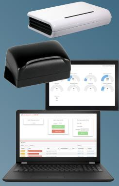
Nexcomm System's SensePoint Commercial Sensor Hub has twelve inputs that can accept any sensor that has a 0 to 5V output, whether it is analog, pulse train or digital on / off. The user can configure the update time base as well as maximum and minimum thresholds for exception reporting. The sensor ADC values are transmitted via an integrated BLE radio.
