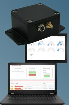
The SensePoint CAN is a very small device that has a CAN interface for monitoring and transmitting messages on a bus with controllers and devices. It has up to 32 message filters to identify specific messages for monitoring. Messages can be sent from the Cloud server for transmission on the bus. A Thread radio wirelessly connects the SensePoint CAN to one of the EdgePoint gateways for communication with cloud servers.
