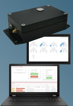
The SensePoint Motor is designed to verify the health of electric motors by monitoring the motor currents and temperatures of various components. It has three 333mV CT channels for monitoring current on each motor phase and eight PT100 RTD channels. A single optoisolated input can monitor contact closures or alerts from the motor. A digital pulse input can monitor switches or pulse sensors, such as flow meters.
