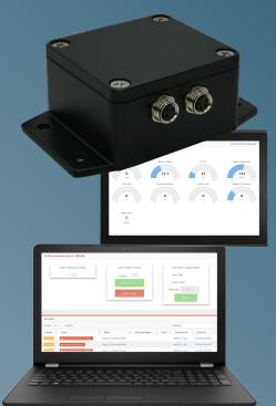
The SensePoint Serial node has one RS-485 and one RS-232 channel for communication to controllers, PLCs, or sensors. It communicates with an EdgePoint Nexus over a customized Thread wireless link. This allows serial commands and data to be passed from a cloud server to the connected device through the Nexus system.
