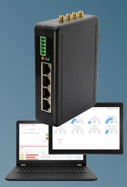
The Nexus Panel is a small cellular gateway designed for industrial panel applications. RS-485 and USB ports allow it to connect to a wide array of PLCs, controllers, sensors, and other equipment for real-time monitoring. A single digital input can be used as an alarm or trigger and a single digital output can be used for signaling external devices. It can accept one of two daughter cards: a 4-port Ethernet switch or an RTD / CT card that is designed for electric motor or pump monitoring.
