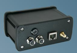
They offer both Ethernet and RS-485 ports to wire to external devices, such as drives, controllers and PLCs. Ethernet is on a standard RJ-45 connector. RS-485 is on a 4-pin M8 connector.
