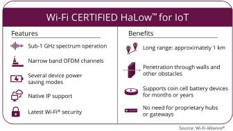
The 802.11ah specification or Wi-Fi HaLow, was released by the Wi-Fi Alliance in 2017. It is best described as "sub-GHz long-range Wi-Fi". It takes the features that have made Wi-Fi one of the most successful wireless protocols and brings it into lower frequency bands. It fills a gap by offering much better range than Bluetooth and IEEE 802.15.4 radios while offering much better data throughput than protocols like ZigBee, Thread and LoRa. This allows it to offer several distinct advantages.
